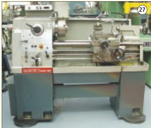
COLCHESTER STUDENT 3100: Centre Lathe. 13" Swing Over Bed. 25" Between Centre. Variable Speed 20-3100 rpm. £3,950
