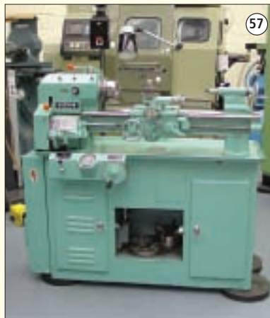
BOXFORD: Centre Lathe. 10" Swing Over Bed. 20" Between Centres. Variable Speed. Norton Gear Box. 3&4 Jaw Chuck. Ex. College. £1,250
