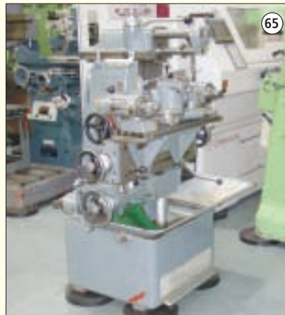
SCHAUBLIN 13: High Precision Universal Mill. Table 600mm x 210mm. Taper 30 ISO. Variable Speed. Very well equipped. £3,250
