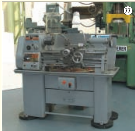
COLCHESTER BANTAM 1600: Centre Lathe. 11" Swing Over Bed. 20" Between Centres. (Ex. College).
