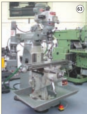
BRIDGEPORT: Turret Mill. Table 42" x 9". Variable Speed Head 1½" HP. Ex. University Ex. Condition. £2,750
