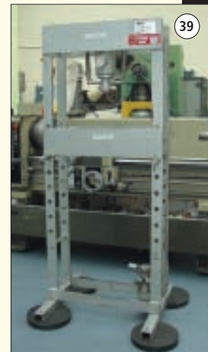
TANGYE Type PR20: 20 Ton Workshop Press. 39" Daylight. 25" Between Frames. £750
