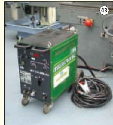
MIGATRONIC Type MTE 220 Dialog: Tig Welding Set. 200 amp AC/DC. £850
