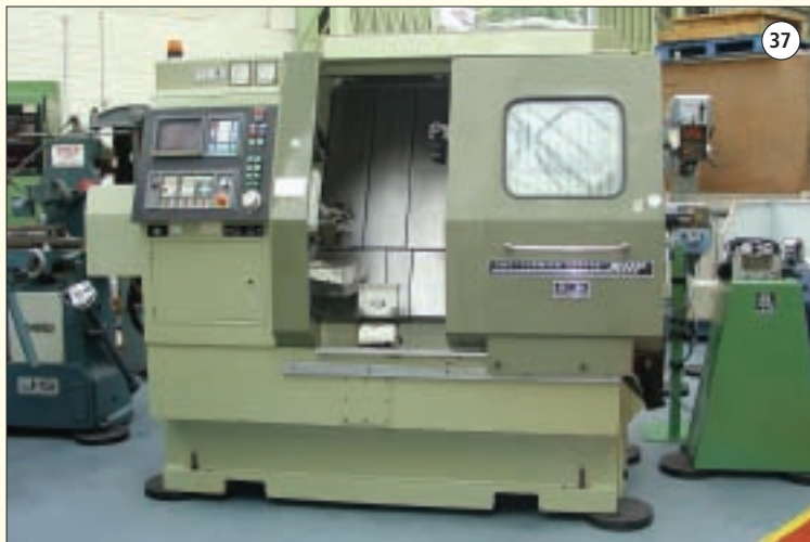
MHP Model MT50: Slant Bed Turning Centre. 450mm Swing Over Bed. 550mm Long Travel. Spindle Bore 60mm. 50mm Bar Cap. 'Live Tooling' 25 HP. Bi-directional Turret. Ex. Univesity.
