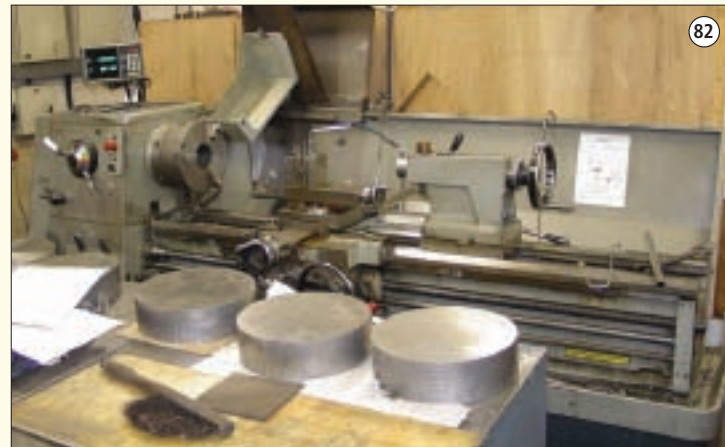
COLCHESTER MASTIFF 1400: Centre Lathe. 21" Diameter Swing Over Bed. 80" Between Centres. Complete With 2 Axis Digital Readout. (Still on Site - Due In Immanently).
