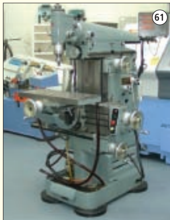
THIEL 159: Precision Toolroom Universal Mill. Tilt & Swivel Table 800 x 270mm. Spindle 40 ISO. With Tooling & 3 axis DRO.
