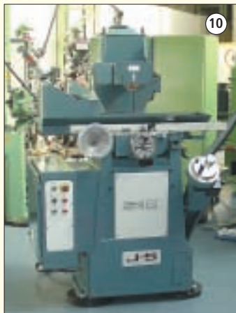
JONES & SHIPMAN: Type 540P Toolroom Surface Grinder. Year 1988. Power Rise & Fall. £4,250
