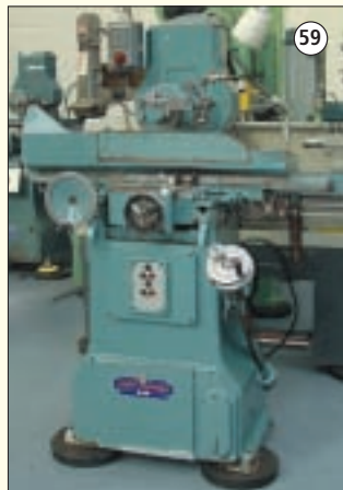
JONES & SHIPMAN 540: Toolroom Surface Grinder. Capacity 18" x 6".
