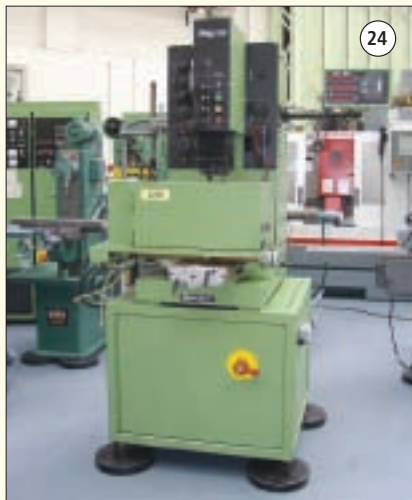
MECRODE NL201 Minor: Spark Eroder. Amps 9+p. 11 kva. Table 425mm x 210mm. Tank 550 x 390mm. With 3 Axis Goodwin Executive 3A-MI D.R.O. £2,950
