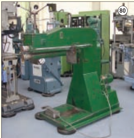
HEAVY DUTY: Power Swager. 37" Throat. 43" Daylight.
