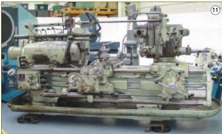
WARD No.8: Combination Turret Lathe. 20" Swing Over Bed. Spindle Bore 3 1/4". Lots of Tooling.
