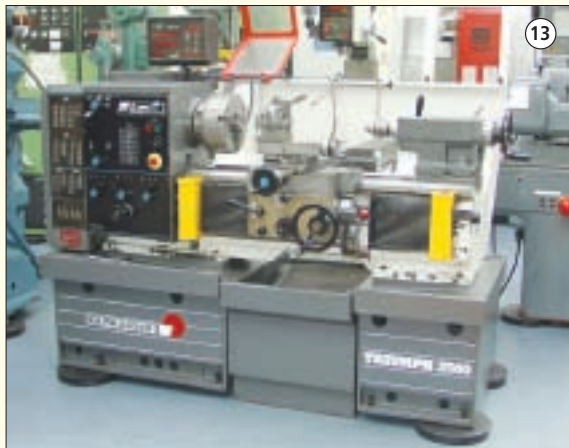
COLCHESTER TRIUMPH VS2500: Variable Speed Centre Lathe. 400mm Dia. Swing Over Bed. 650mm between Centres. Variable Spindle Speeds 14 to 2500 rpm. With D.R.O.
