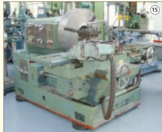
SWIFT Type TB: Copy Facing Lathe. 36" Swing over Bed. 3 1/2" Spindle Bore Width of Gap 13". Speeds 9 to 420 rpm. Complete with Hydraulic Copying & 29" Diameter, 9" Bore 3 Jaw Chuck
