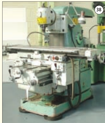
TOS TYPE FA4AU: Universal Miller. Table Size 1600mm x 350mm. Longitudinal Traverse 1000mm. 50 ISO Taper. Speeds 32 to 1400 rpm. Swivelling Vertical Head. £4,750
