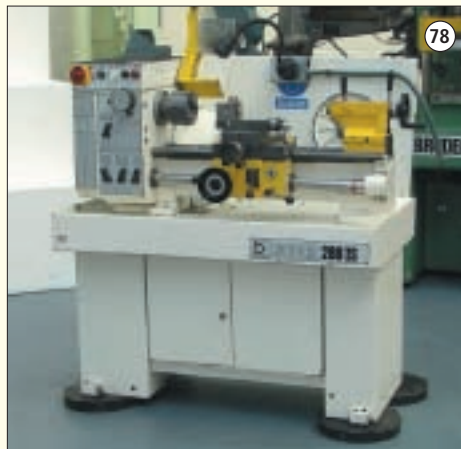
COLCHESTER BOXFORD 280 IS: Centre Lathe. 280mm Swing Over Bed. 500mm Between Centres. Speeds 40 – 2240rpm. £1,500
