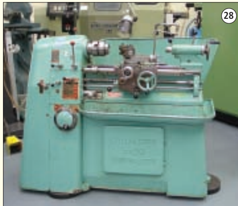
COLCHESTER Chipmaster: Centre Lathe. 10" Swing Over Bed. 20" Between Centres. 1½" Spindle Bore. £950
