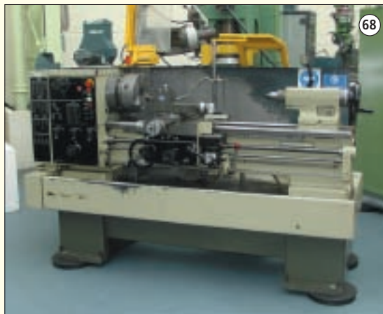
HARRISON M350: Centre Lathe. 380mm Swing Over Bed. 1000mm Between Centres. 54mm Spindle Bore. Speeds 40-2200 rpm. Dual Dials. Metric Screw Cutting. Ainst Threading. 3&4 Jaw Chucks. Q.C.T.P. £4,750
