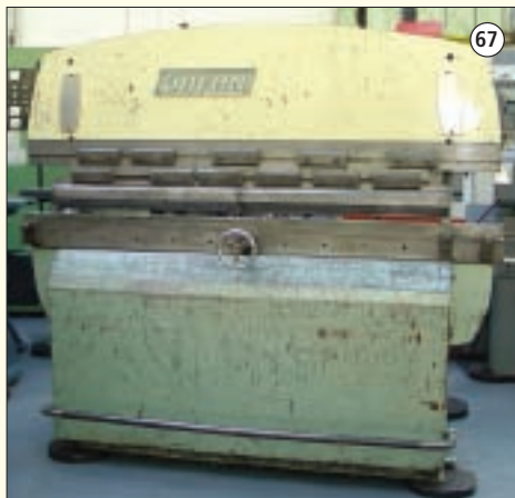
SAFAN Type 50-2000: Hydraulic Upstroke Brakepress. Cap 50 Ton x 2m. Front Operated Back Gauge.
