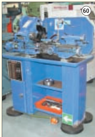
MYFORD Super 7B: 5" Swing over bed. 20" B/C. Norton Box. Power Cross Feed. Ex MOD.
